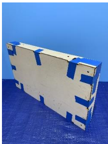
The CMR T-TRAK box is assembled, glued, and taped while the Tite-Bond glue dries.
