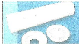
PVC pipe and test caps
